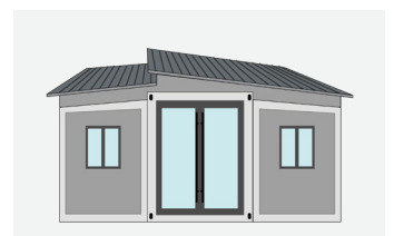
Double slope roof
